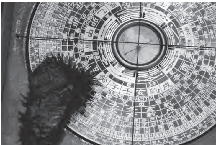
Luopan needle attracted to a piece of magnetite.
