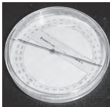
Compass made in laboratory class, white mark on needle indicates south.
