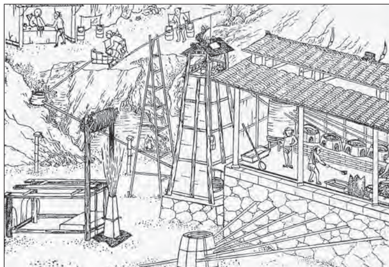
A sketch originally from The Annals of Salt Law of Sichuan Province . A "Kang Pen" drum is seen in the center foreground, with gas pipes feeding the salt stoves in the open building. At the top, brine from a remote well is being carried in buckets by men, who feed it into a bamboo pipeline that runs down to the stoves (from Zhong & Huang). Source: "Ancient Chinese Drilling" by Oliver Kuhn on the Recorder website at http://tinyurl.com/hbdcxea .
